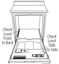
· Level the dishwasher by adjusting the four leveling legs individually.
